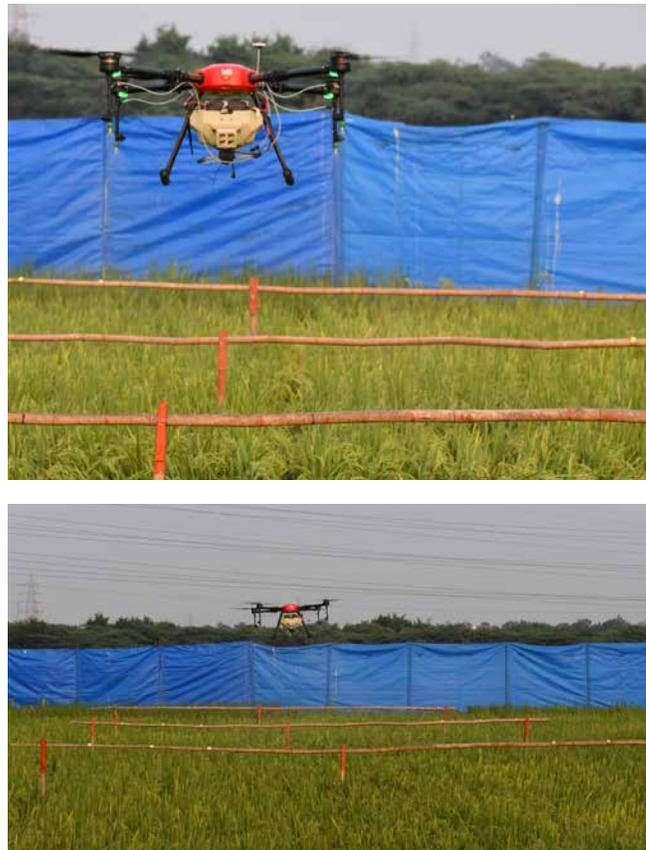
**Fig. 6.8 Placement of water sensitive papers at each sampling position for measuring spray swath width**
