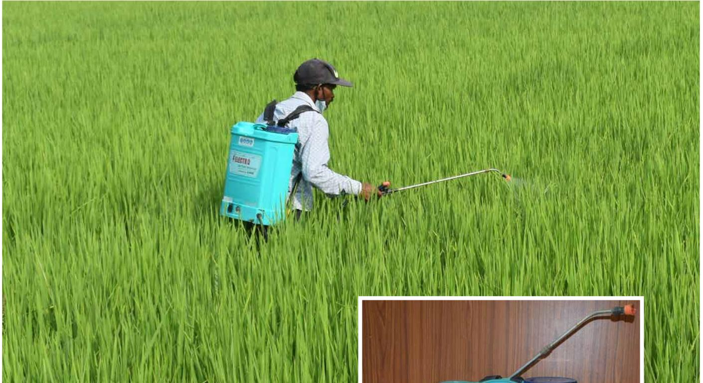
**Fig.6.16 Knapsack electro battery sprayer for manual spraying**
