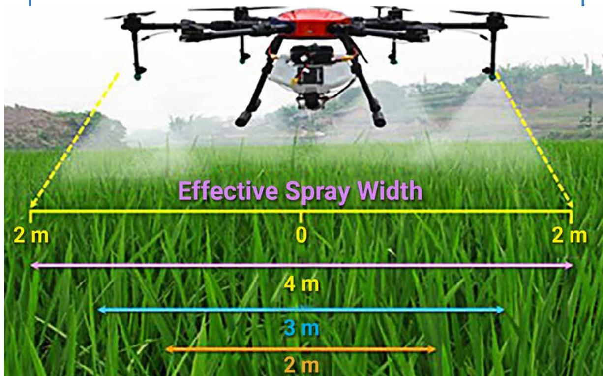
Fig. 6.9 Measuring of spray swath width
