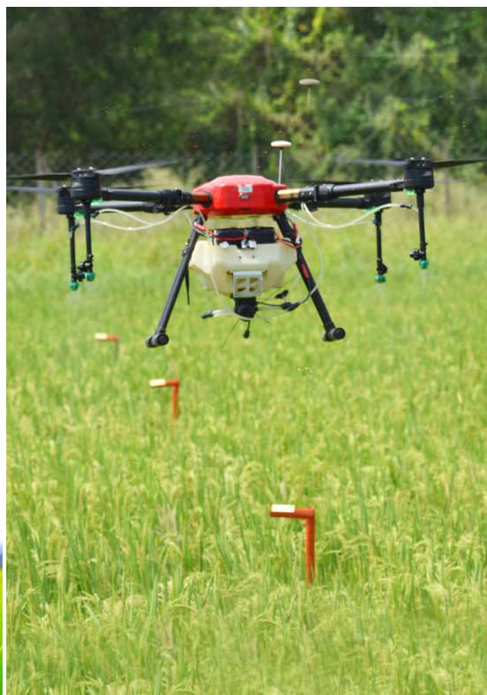
Fig. 6.7 Placement of water sensitive papers at each sampling position within paddy canopy for measuring the droplet parameters
