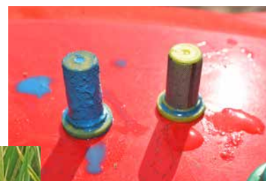
Clogging of nozzle filters
