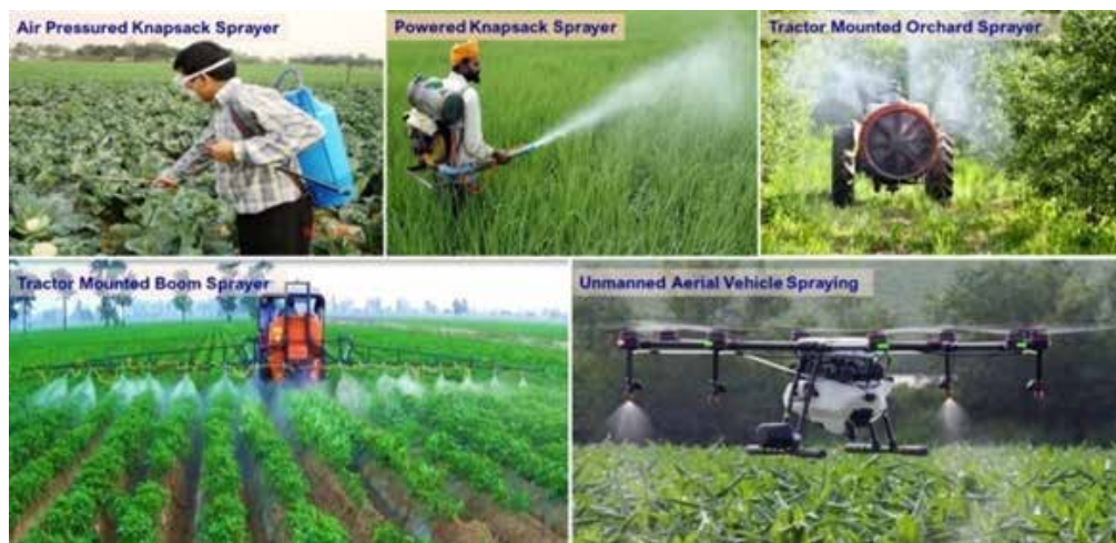
Fig. 3.1 Spraying equipment for pest control used in India and Unmanned Aerial Vehicle spraying
